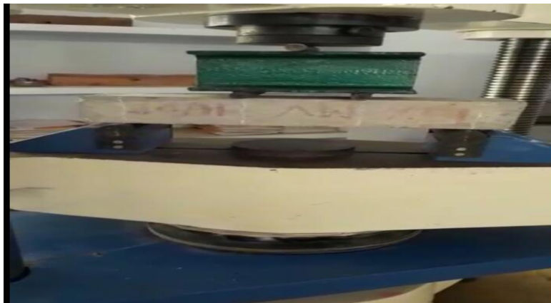
Fig. 4: Flexural strength testing set up
