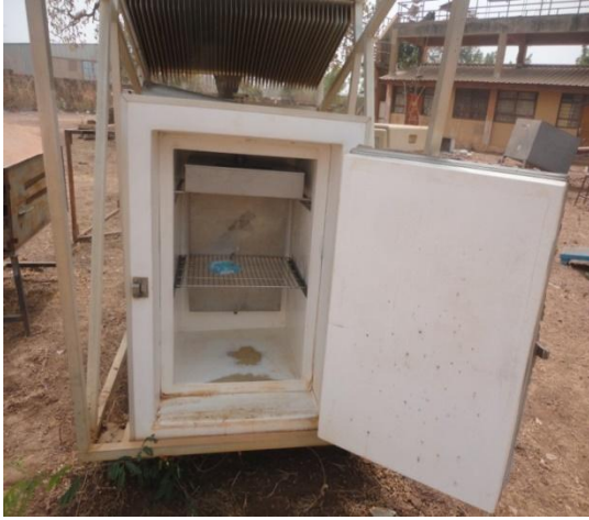
Figure 1 : Photo of the evaporator and the chest
